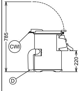
CWI1 = D = Cold Water inlet 1 Drain
